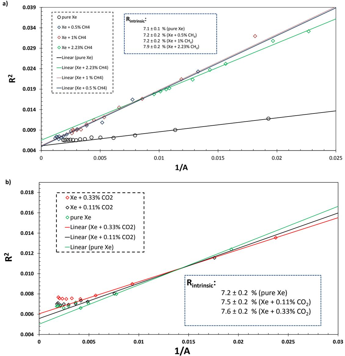
**Figure 9:** Dependence of  $R^2$  on  $A^{-1}$  for the present GPSC, for the different Xe+CH<sub>4</sub> mixtures (a) and different Xe+CO<sub>2</sub> mixtures. As expected, a linear trend is observed for a certain range of amplitudes.
