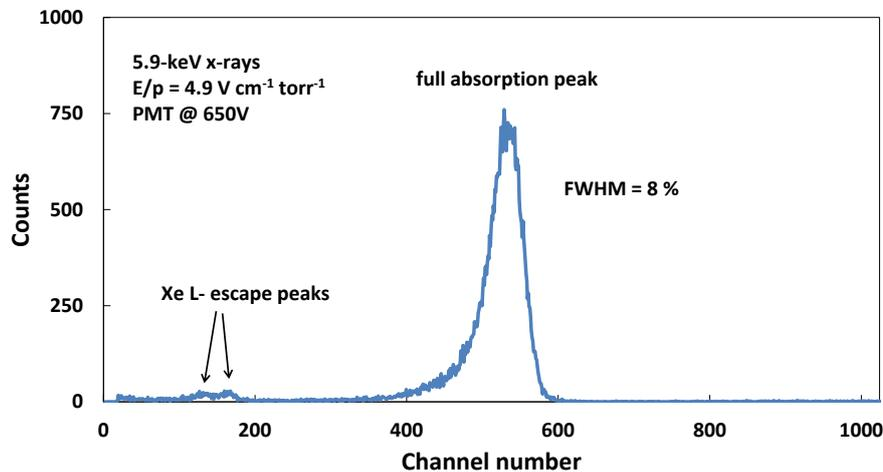
**Figure 3:** Pulse-height distribution for 5.9-keV x-rays absorbed in the xenon driftless GPSC. The PMT was biased at 650 V, the reduced electric field was  $4.9 \text{ V cm}^{-1} \text{ torr}^{-1}$  and formatting constants were  $5 \mu\text{s}$ .
