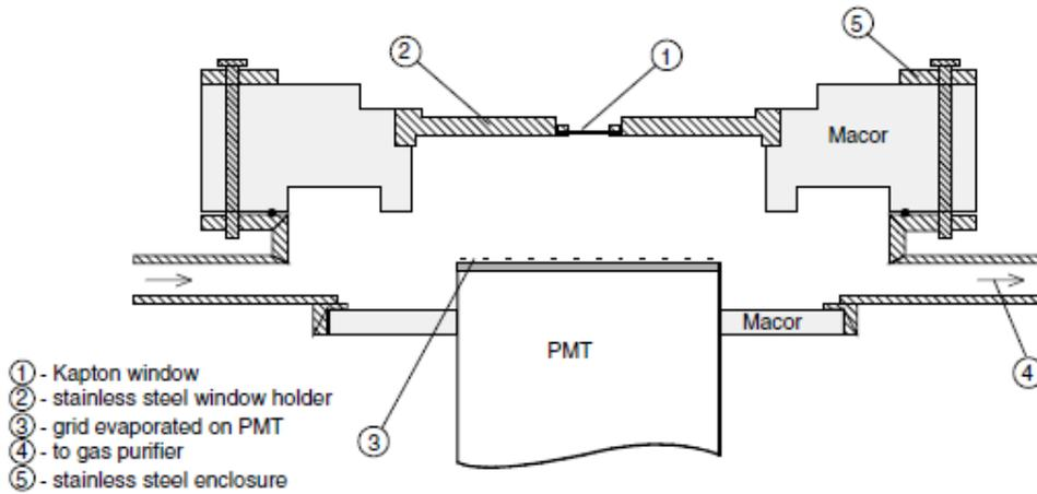
**Figure 1:** Scheme of the driftless GPSC used in this work [3].
