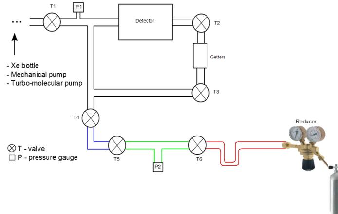
**Figure 2:** Scheme of both gas systems connected to the detector.
