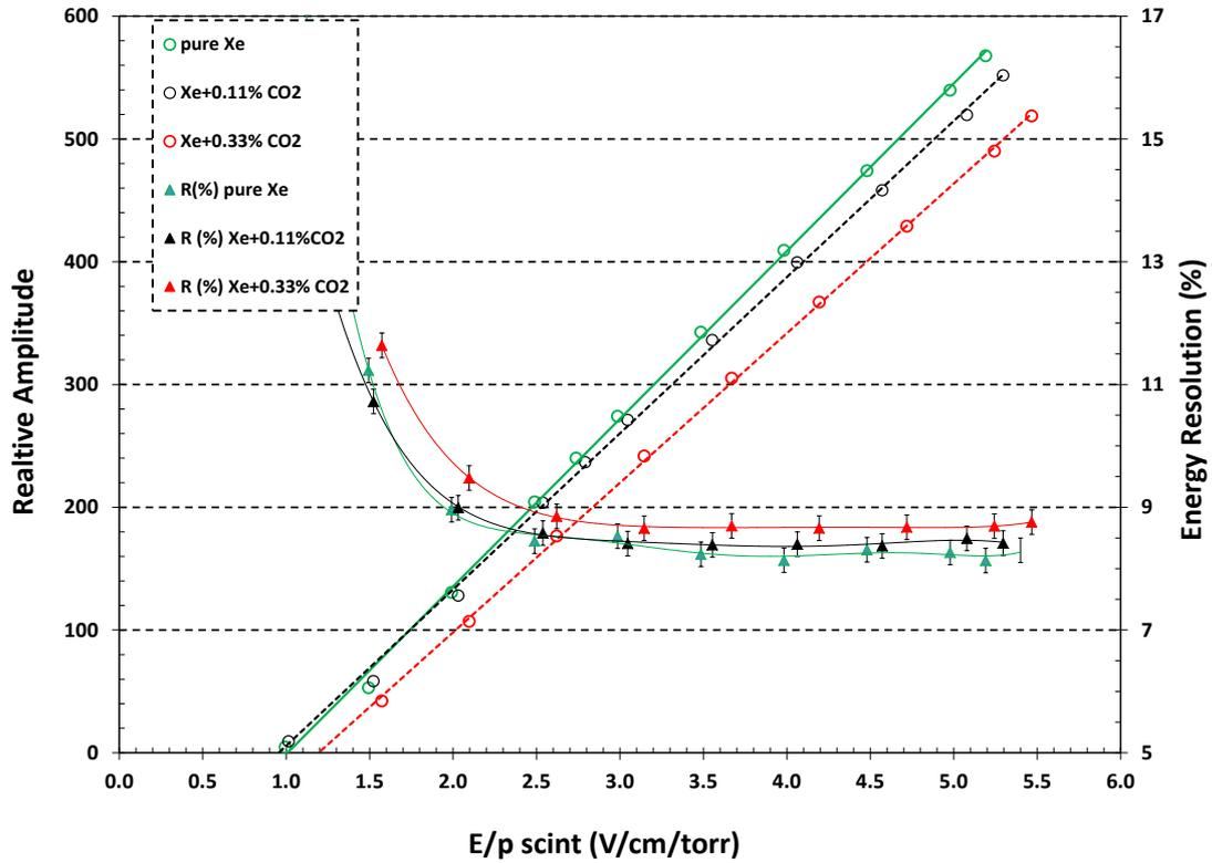
**Figure 6:** Relative amplitude as a function of reduced electric field,  $E/p$ , for pure xenon and for the mixtures of 99.89% Xe+0.11% CO<sub>2</sub> and 99.67% Xe+0.33% CO<sub>2</sub>, for getters operating at 80°C, a constant PMT bias voltage of 650 V and shaping constants of 5  $\mu$ s.
