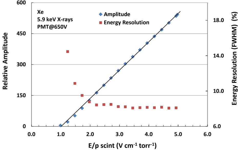
**Figure 4:** Relative amplitude and energy resolution (FWHM) as a function of reduced electric field,  $E/p$ , for pure xenon, for 5  $\mu s$  shaping constants. A PMT bias voltage of 650 V was used and the gas pressure was 800 torr.
