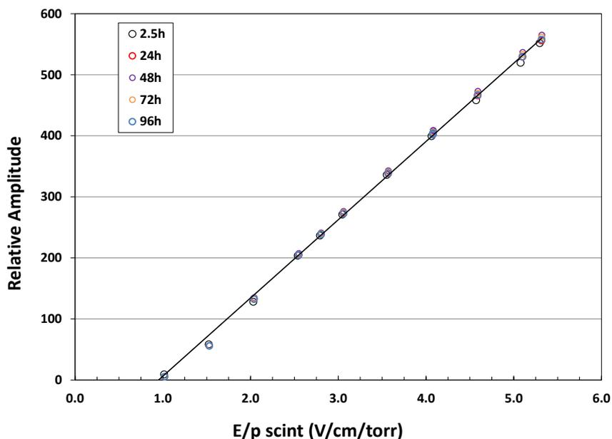
**Figure 5:** Relative amplitude as a function of reduced electric field,  $E/p$ , for the mixture of 99.89% Xe+0.11% CO<sub>2</sub> at 80°C with a filling pressure of 750 torr, for a constant PMT bias voltage of 650 V and shaping constants of 5  $\mu$ s.
