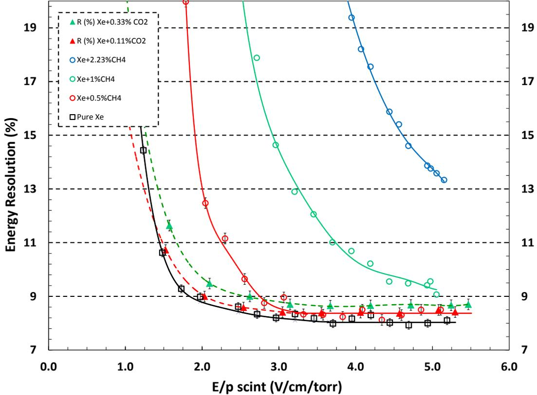
**Figure 8:** Energy resolution (FWHM) as a function of reduced electric field in the scintillation region, for pure xenon and for the Xe-CH<sub>4</sub> and Xe-CO<sub>2</sub> mixtures studied in this work. The lines serve only to guide the eye.
