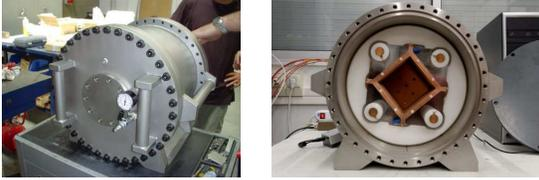
Figure 1. Left picture shows the aluminum pressure vessel of the TPC. Right picture shows the inner structure of the TPC can be seen.
